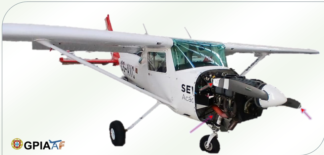
Detalhe dos danos na aeronave || Detail of aircraft damage
